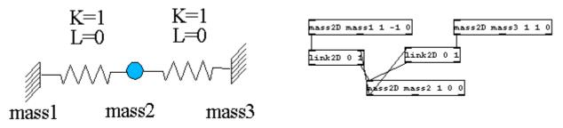
Figure 7: a small system, and it's equivalent using pmpd and pd
