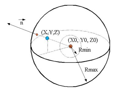
Blue point is a mass, red point is the center of the iSphere3D Figure 18: iSphere3D
